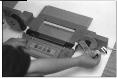
Thread film under the white guide rollers, between the glass flats to the quick take up reel.
